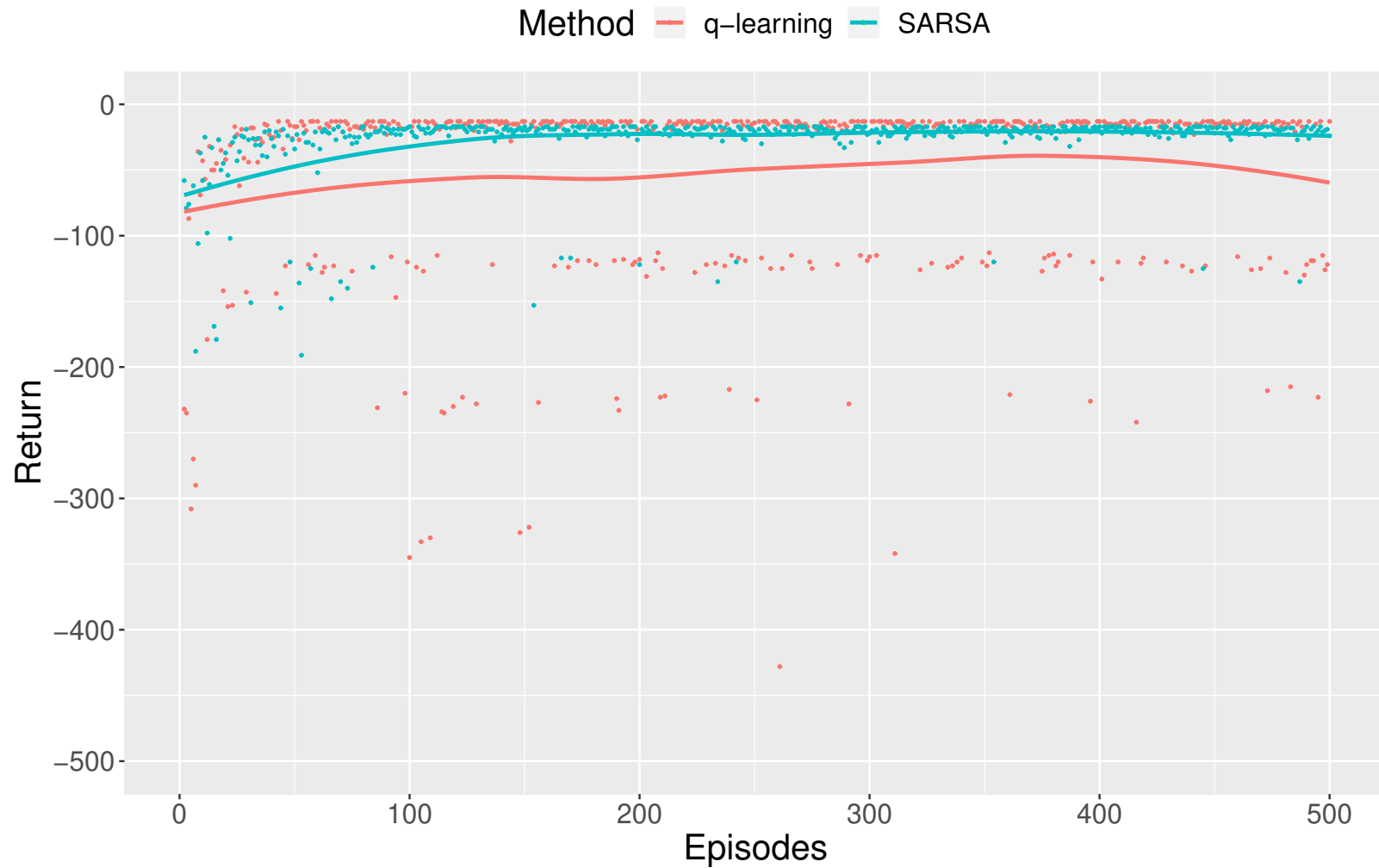
Figure 12: Performance of the SARSA and q-learning learning algorithm on the Cliff example. Settings: discount factor \gamma = 1 , exploration rate \varepsilon = 0.1 and step size \alpha = 0.5 .
